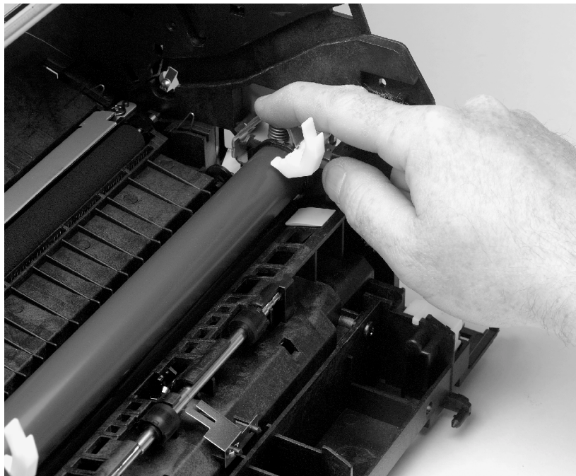
Figure 47. Fusing element metal clips reinstallation
