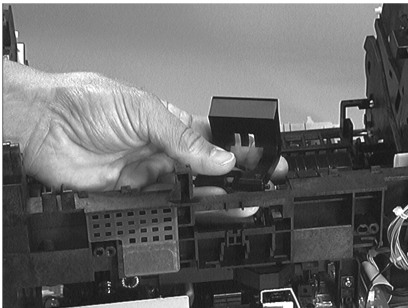
Figure 62. Separation pad removal (2 of 2)
