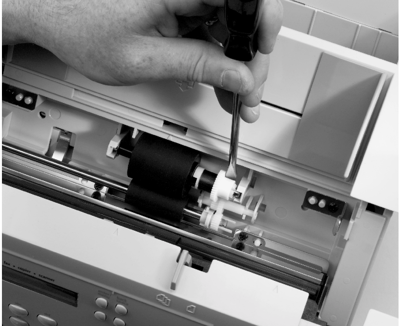
Figure 32. Document scanner pickup roller removal
